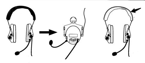
**STEP 1**Free the headband cable that connects the two ear shells by removing the Velcro headband cloth.
